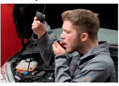
Set the tester down vertically on the palm of your hand and breathe into the intake opening: exhale deeply and slowly, actuating the suction ball once or twice only.
