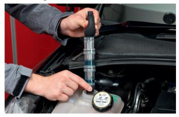
Keep the tester ready with the fluid adjusted **blue-green**. Open the lid of the expansion tank of the cooling system and insert the tester immediately in order to prevent the escape of any combustion gases that may be present. Examine the cooling system for the presence of increased  $CO_2$  content by pumping the suction ball about 5 times.
