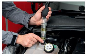
If the air pocket contains combustion gas (increased  $CO_2$  content), the test fluid will be discolored towards **yellow** (= **leak**).
