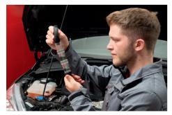
Finally, by actuating the suction ball several times and taking in fresh air, regenerate the fluid in both chambers until it turns blue-green (enhanced reaction sensitivity).
